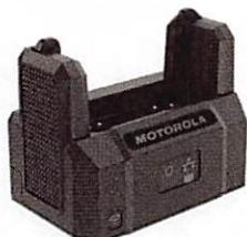
**Wi-Fi Base** - The Wi-Fi Base is mounted in the vehicle. It facilitates V300 upload of evidence to evidence management system, firmware updates, communication between V300 and in-car group devices, charges fully assembled V300 cameras or individual battery packs and more. It has LED indications of battery charging status and upload, and an ambient light sensor for optimal LED brightness control, from the bright sunlight, to the dim interior of a patrol car.
